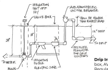
**Drip Irrigation Valve:** Irrigation Shut Off, valve in valve box, AVB Automatic Vacuum Breaker and Pressure Regulator.
